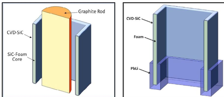
Fig. 5. CAD solid models of the FCI segments for thermo mechanical analysis. (Left) for inductively heating test. (Right) for PbLi submersion test.
