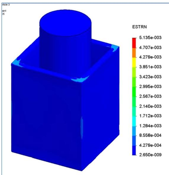
Fig. 10. Simulated strain contours of the inductively heated FCI segment.
