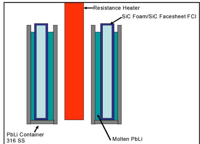
Fig. 4. Schematic of the FCI prototype liquid-PbLi testing apparatus.
