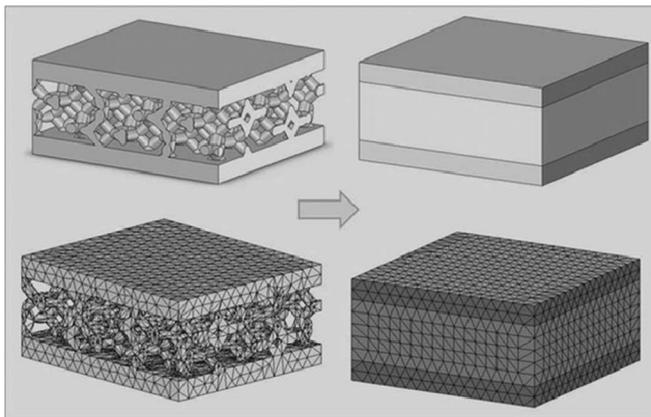
Fig. 6. Detailed (top) 3-D solid and (bottom) meshed model of a section of the open-cell SiC-foam FCI structure (wall: ~1 mm; foam: ~3 mm thick). (Right) FCI wall model represented by homogeneous materials.
