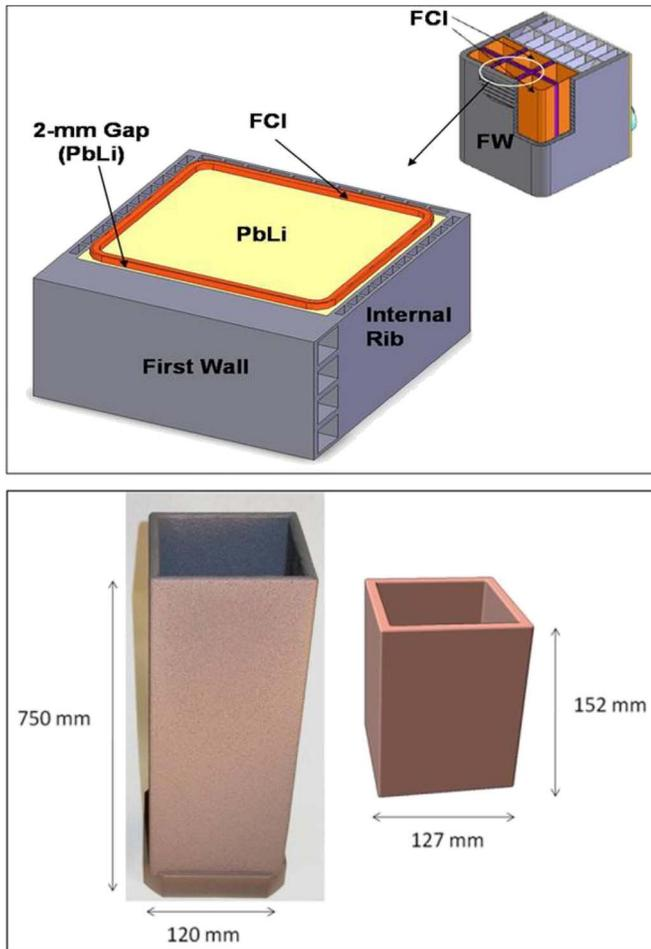
Fig. 1. (Top) Model of a DCLL ITER TBM section, showing the location of the FCI inside the TBM (TBM full height:  $\sim 1.66$  m). (Bottom) (Left) Full-scale FCI prototype and (right) CAD model of the heat-tested FCI segment.
