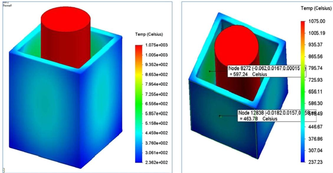
Fig. 8. Simulated steady-state temperature contours of the radiatively heated inner walls (note the uneven temperature distribution along the FCI inner and outer walls).
