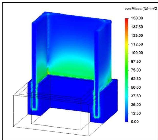
Fig. 12. Von Mises stress contours across the FCI prototype structure.
