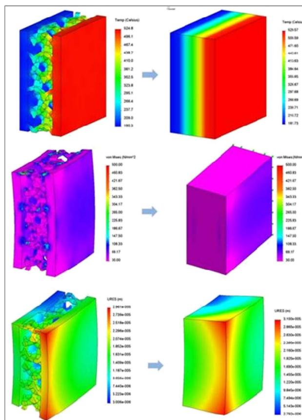
Fig. 7. FEM analysis of the detailed foam geometry for establishing the homogeneous material properties of a surrogate SiC-foam material: (Top) Temperature, (middle) von Mises stress, and (bottom) displacement.
