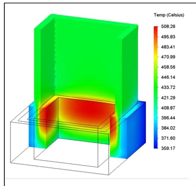
Fig. 11. Temperature contours in the FCI prototype structures for a  $\Delta T$  of about 150 °C between the ID and OD of the FCI.
