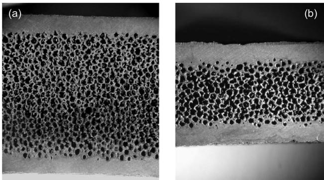
Fig. 2. (a) Cross-sectional photograph of a 10-mm-thick 12% dense SiC foam (100 ppi) with 1.8-mm-thick CVD SiC face sheets. (b) Photograph of a 5-mm-thick 22% dense SiC foam (100 ppi) with 1.8-mm-thick CVD SiC face sheets. Both  $5 \times$ . (Ultramet, Inc.).
