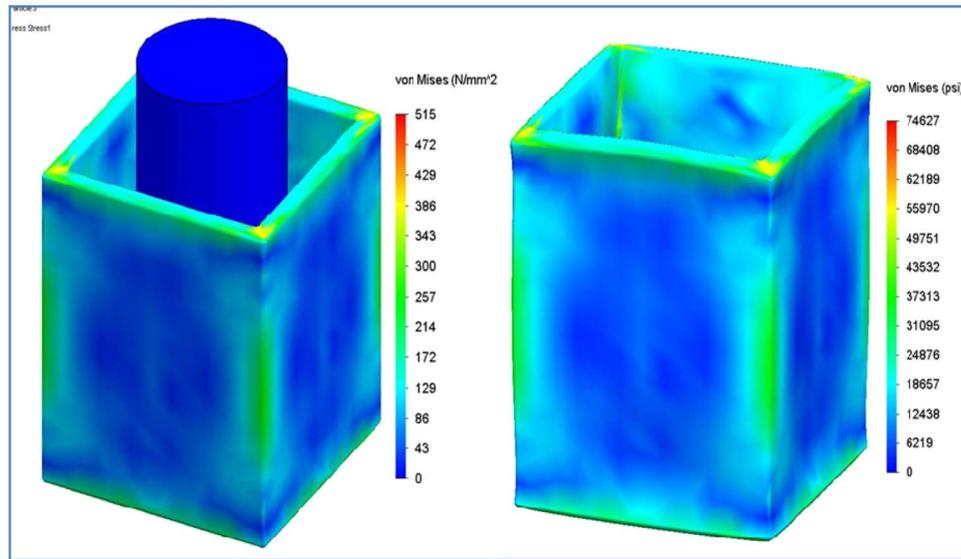
Fig. 9. Von Mises stress contours of the (left) FCI-graphite-rod assembly and of the (right) FCI prototype alone with a scaled up deformation (100 ×). Note the difference in units.
