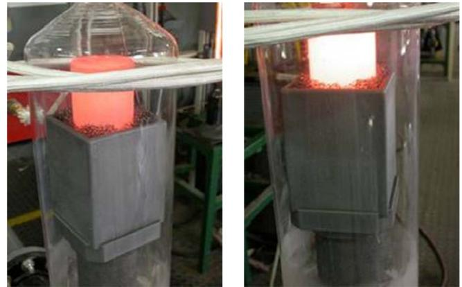
Fig. 3. Photographs of the inductive heat testing of a 0.15-m-tall FCI segment at (left) intermediate ( $\sim 200$  °C ID) and (right) high ( $\sim 600$  °C ID) temperatures (Ultramet, Inc.).
