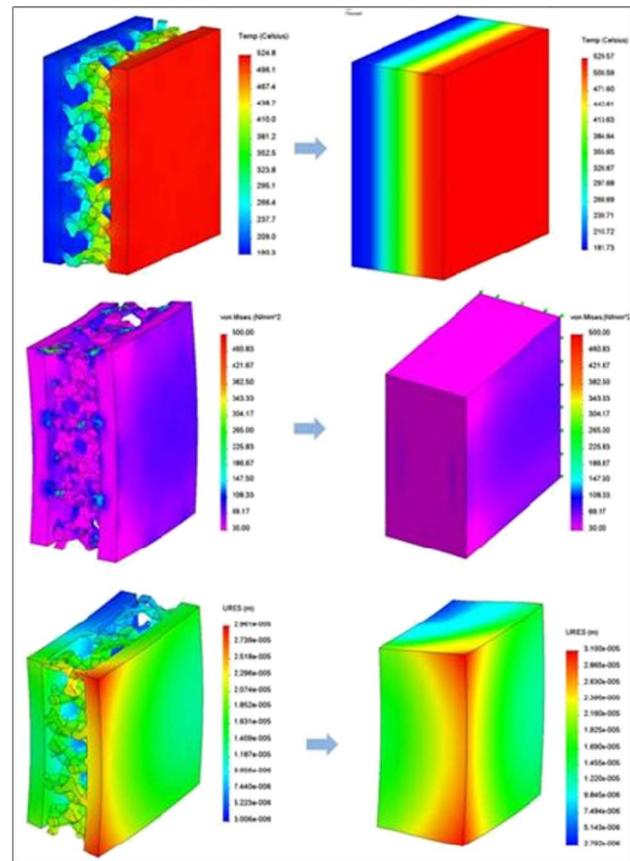
Fig. 7. FEM analysis of the detailed foam geometry for establishing the homogeneous material properties of a surrogate SiC-foam material: (Top) Temperature, (middle) von Mises stress, and (bottom) displacement.
