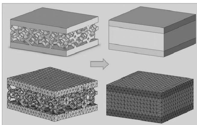
Fig. 6. Detailed (top) 3-D solid and (bottom) meshed model of a section of the open-cell SiC-foam FCI structure (wall:  $\sim 1$  mm; foam:  $\sim 3$  mm thick). (Right) FCI wall model represented by homogeneous materials.
