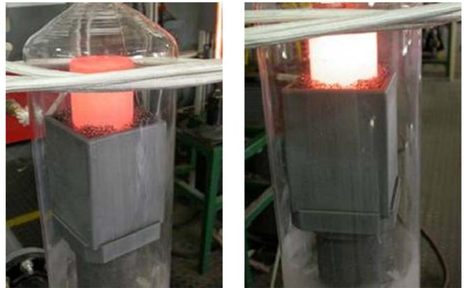
Fig. 3. Photographs of the inductive heat testing of a 0.15-m-tall FCI segment at (left) intermediate ( $\sim 200$  °C ID) and (right) high ( $\sim 600$  °C ID) temperatures (Ultramet, Inc.).
